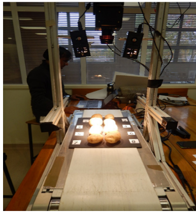
Figure 2. Potatoes Hyperspectral Image capturing on moving belt
