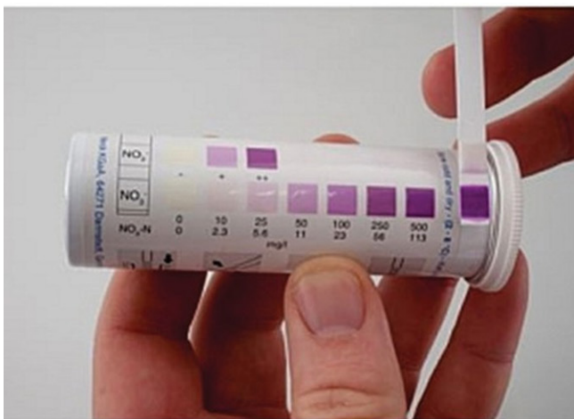
Test strip used to determine available N in a soil sample
