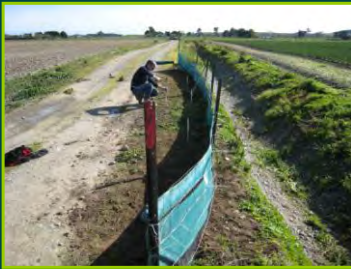
Picture: Field tests of sediment movement on dairy land converted to brassica production in the Horowhenua district
