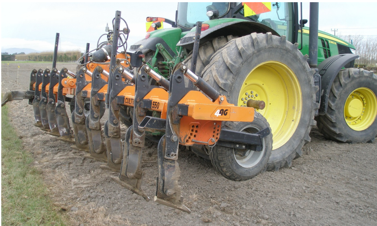
Figure 2. Sub-soiler used to apply a sub-soil tillage down to 370 mm on half of the plots.
