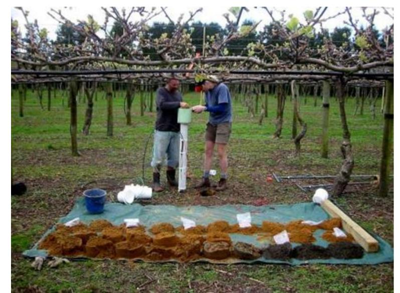
12 fluxmeters/site Measuring; Soil water flow in mm/day and Leaching losses NH<sub>4</sub><sup>+</sup> and NO<sub>3</sub><sup>-</sup>
