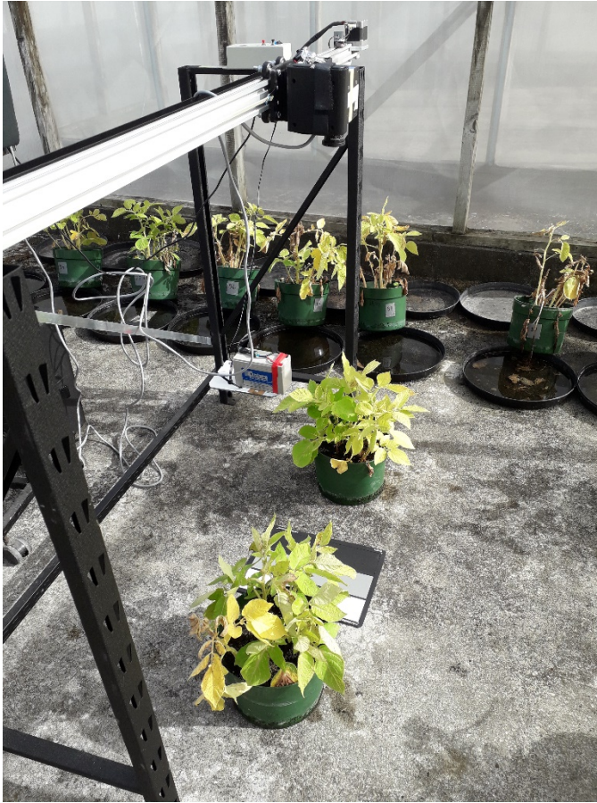
Figure 1 A Headwall Photonics Nano hyperspectral camera mounted on automated gantry system. The camera slides along the rail at a velocity proportional to the amount of incident light. Potato plants were scanned in pairs. A single scan of the plants collected a hyperspectral 'cube' consisting of 800 lines of 640 \text{ pixels} \times 274 \text{ spectral bands} . The card lying between the plants acts as a reference to convert radiance into reflectance.
