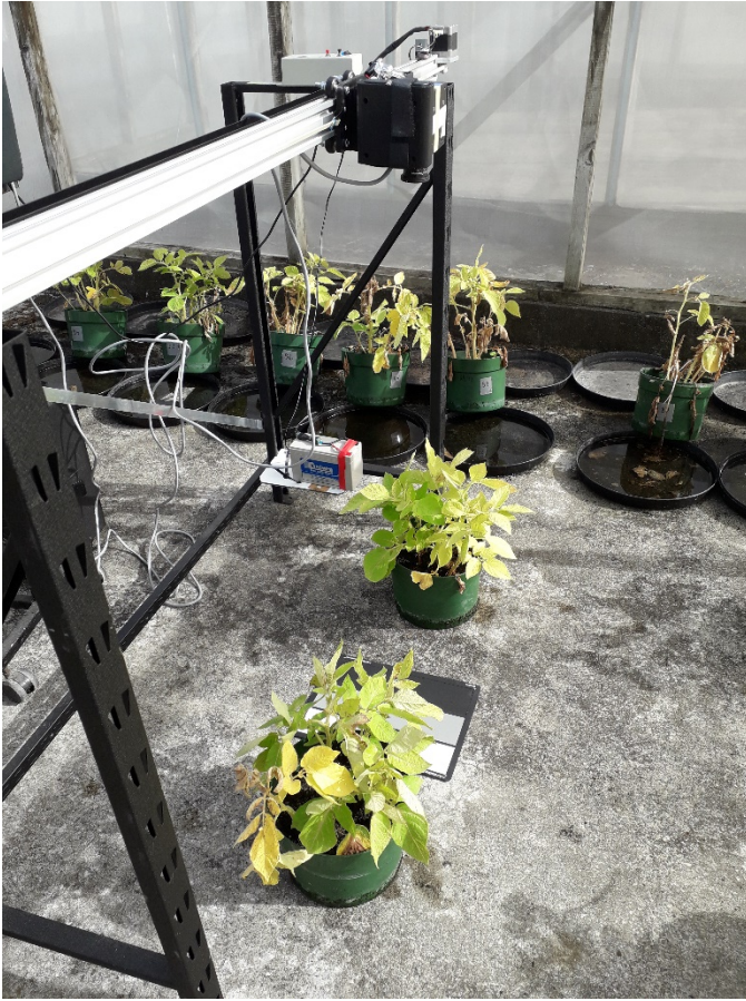
Figure 1 A Headwall Photonics Nano hyperspectral camera mounted on automated gantry system. The camera slides along the rail at a velocity proportional to the amount of incident light. Potato plants were scanned in pairs. A single scan of the plants collected a hyperspectral 'cube' consisting of 800 lines of 640 pixels \times 274 spectral bands. The card lying between the plants acts as a reference to convert radiance into reflectance.
