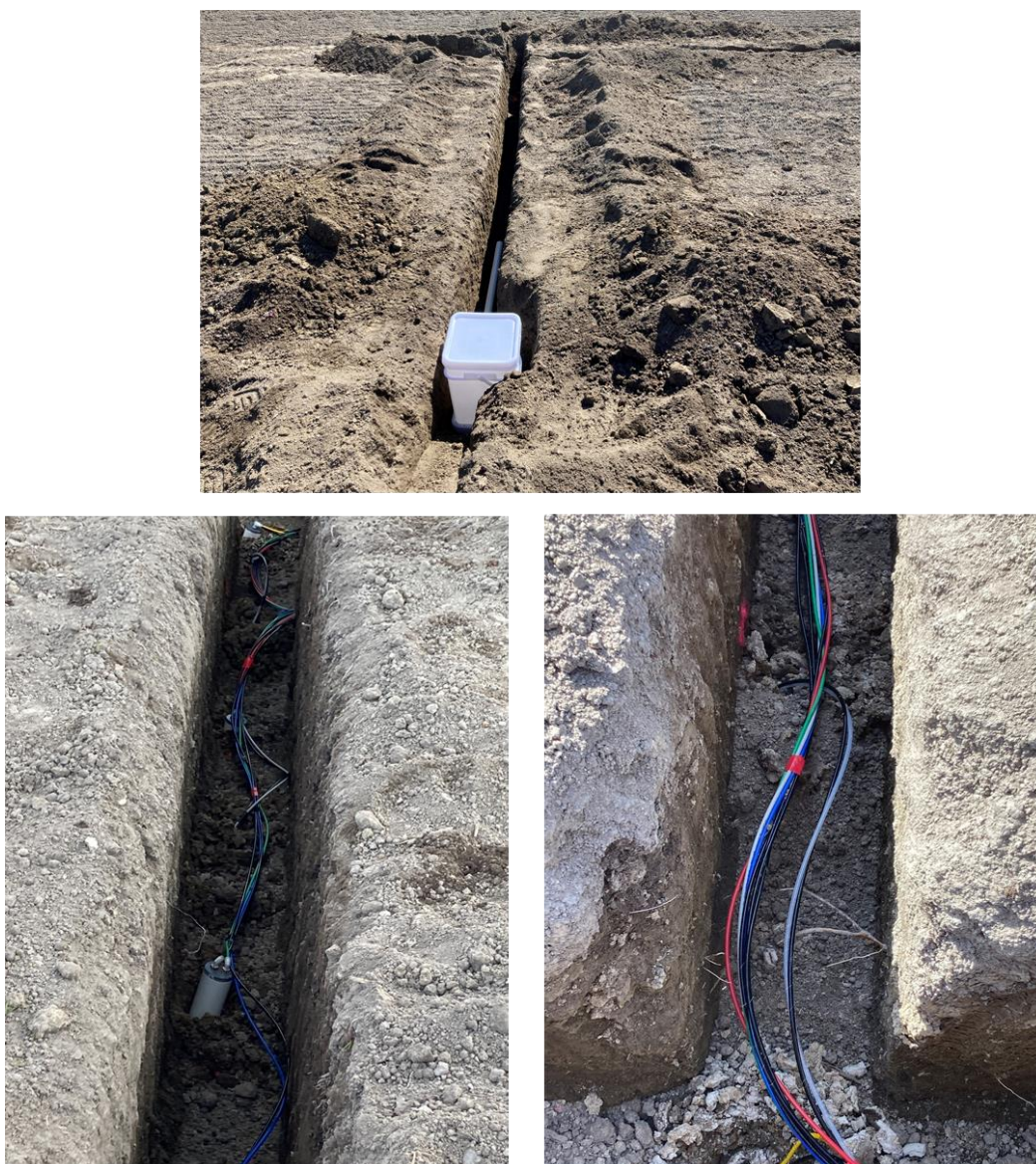
Figure 15. Suction cup installation. Clockwise from the top, shows the trenches set up to connect the suction cup via tubes to a sampling sump. During crop growth, the sump is located at soil surface level for access. During cultivation, the top portion of the sump is removed and the lower portion buried. Tubes from suction cups along trench floor, and views of suction cups in soil and tubes leading from them towards the sump and sampling point.
