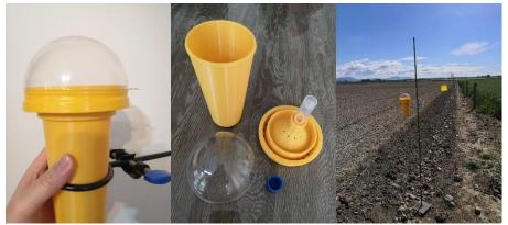
The concept is to trap predominantly psyllids and less other species, so as to make collection and identification easier. The trap uses antifreeze in the test tube to preserve the insects. The collector then puts a cap on the tube when collecting it and replaces it with a new clean tube. The trap also has the option of holding a psyllid attractant/lure in future, when we have further developed an effective one.
