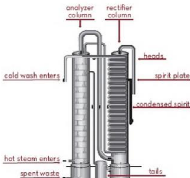
Figure 3- Column Still for continuous fermentation. Source: (Abou-Ganaim, 2013)
