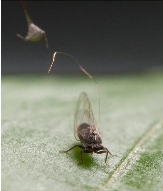
Figure 3. An adult psyllid attached to 10 \mu\text{m} diameter gold wire using conductive silver paint for EPG recording.
