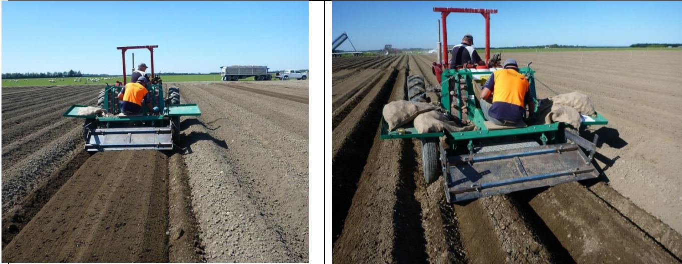
Figure 1. Formation of two row flat-bed (left) and flat-top bed (right, using a modified Grimme planter).
